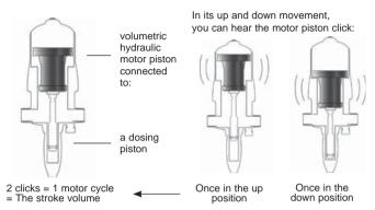
The speed of the motor is proportional to the flow of water passing through the system.
