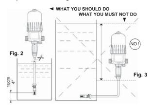
Under no circumstance should the solution level be above the water inlet of the DOSATRON (to avoid siphoning situations) (Fig. 3).
